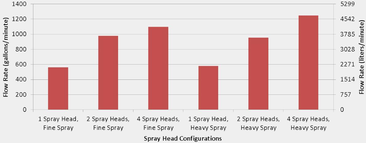
Total flow rates of different spray head configurations. The approximate total flow rates in gallons/minute (left vertical axis) and liters/minute (right vertical axis) of four possible spray head configurations. The “fine spray” opening is ¼ inches in height, and the “heavy spray opening” setting is ¾ inches in height. These flow rates were recorded on an MST8 CAT621K with an M-4B Mega water pump.
