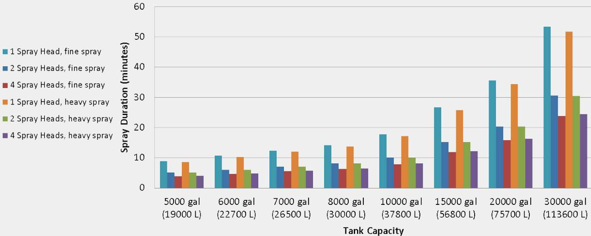
Estimated spray duration for various capacity tanks with four different spray head configurations. Spray duration in minutes is shown on the vertical axis. The “fine spray” opening is ¼ inches in height, and the “heavy spray opening” setting is ¾ inches in height. These flow rates were recorded on an MST8 CAT621K with an M-4B Mega water pump.
